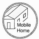
When installed in a mobile home, the heater must be bolted to the floor, have outside air, and NOT BE INSTALLED IN THE BEDROOM (Per H.U.D. requirements). Check with local building officials.
