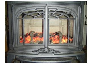
Let the stove burn with the bypass and air control open for about 45 minutes to establish a good coal bed (3" to 4").
