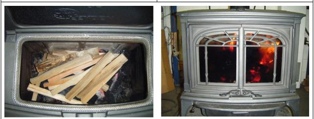
After 13.5 hours you can re-start the fire by opening the bypass and air control and placing some kindling in the stove. After the fire starts burning you can load more wood and repeat the burn process. The glass may become dirty on low burn. By burning on high, with a hot stove, the glass will become clean.
