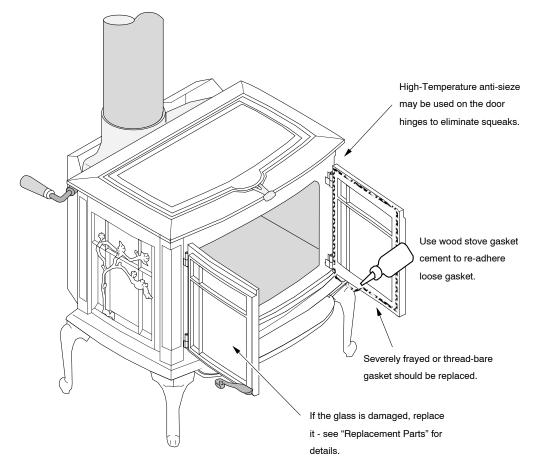
The door latch should pull the door against the face of the stove (but not so tight as to not allow full handle rotation). To adjust the door latch, adjust the position of the striker plate that attaches to the front plate of the stove.
