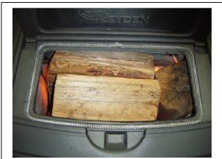
Now that the unit is hot and has a good coal bed, fill the unit with wood, wait a few minutes then close the bypass and adjust the air control to low.
