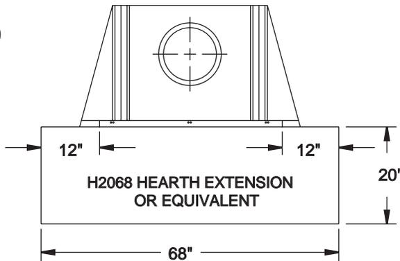
**NOTE:** A hearth extension placed on a combustible floor must be constructed with rigid insulation which has a minimum "R" value of 1.16 or a "K" value of 0.43. The insulation must be covered with a non-combustible covering such as a tile stone, marble, or a piece of 0.018 minimum sheet metal which is needed to protect the insulation. Follow instructions provided with the fireplace for all other specifications and directions for proper installation of the fireplace and hearth extension.
