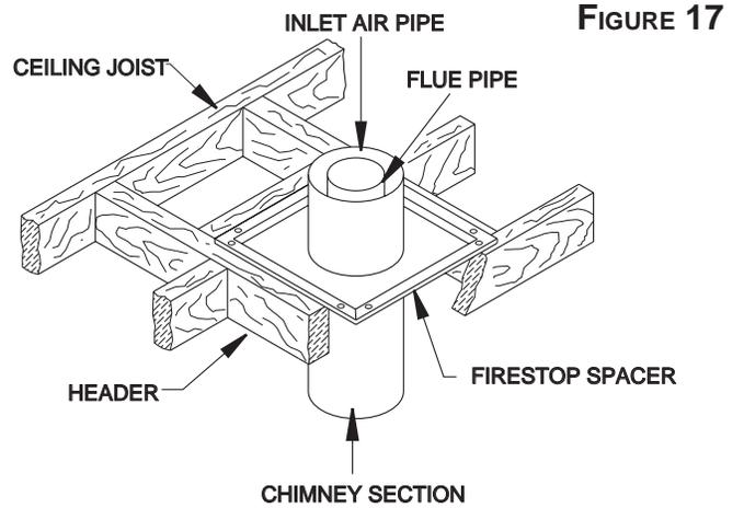
INSTALLATION OF FIRESTOP-SPACER AT FLOOR LEVELS
