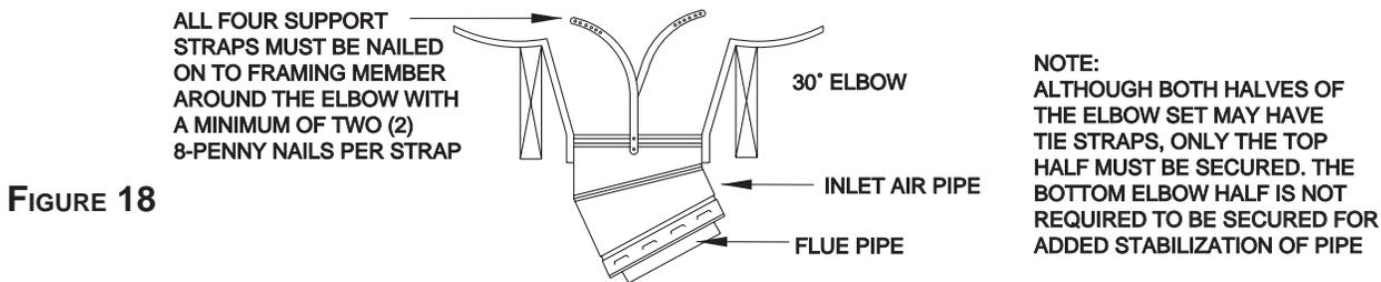
3. The limitations on the quantity of elbows per chimney are as follows: If the total height of the fireplace and chimney is—12' - 2" or more — two elbows may be used in the chimney. 21' - 0" or more — four elbows may be used in the chimney.
