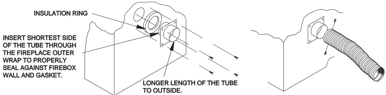
**STEP 1:** SECURE OUTSIDE AIR STARTING COLLAR TO LEFT SIDE OF FIREPLACE WITH FOUR SHEET METAL SCREWS PROVIDED.
