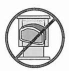
The viewing door and ashpan must be closed and latched during operation.
