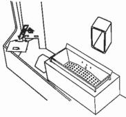
Silde the ash pan trap door forward to expose the ash dumps (the door can be removed and cleaned if necessary)
