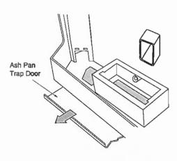
Replace the ash trap doors and firepol. Silde the ash pan trap door forward.
