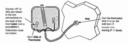
Pull the cover off the thermostat. Place the thermostat in location and attach it to the wall through the two obround holes (use the appropriate screws for the type of wall it is being attached to). Replace the cover on the thermostat to complete the installation.
