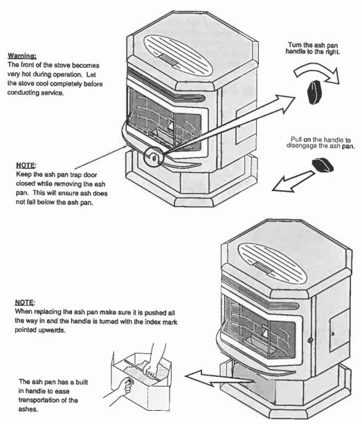
Disposal of Ashes – Ashes should be placed in a metal container with a tight fitting lid. The closed container of ashes should be placed on a noncombustible floor or on the ground, well away from all combustible materials, pending final disposal. If the ashes are disposed of by burial in soil or otherwise locally dispersed, they should be retained in the closed container until all cinders have been thoroughly cooled.
