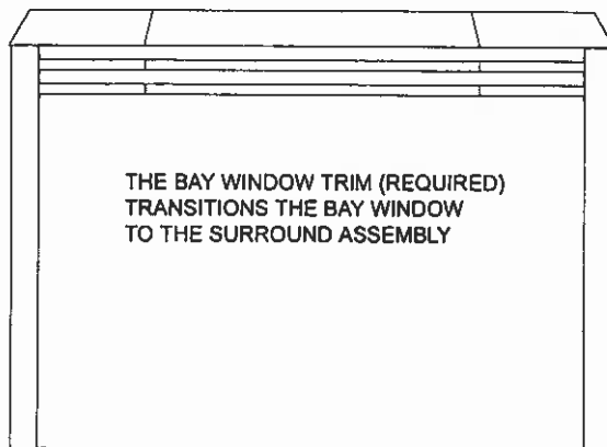
Front View Of Assembled Trim Align the 6 Clips on Trim Back with Surround Pins
