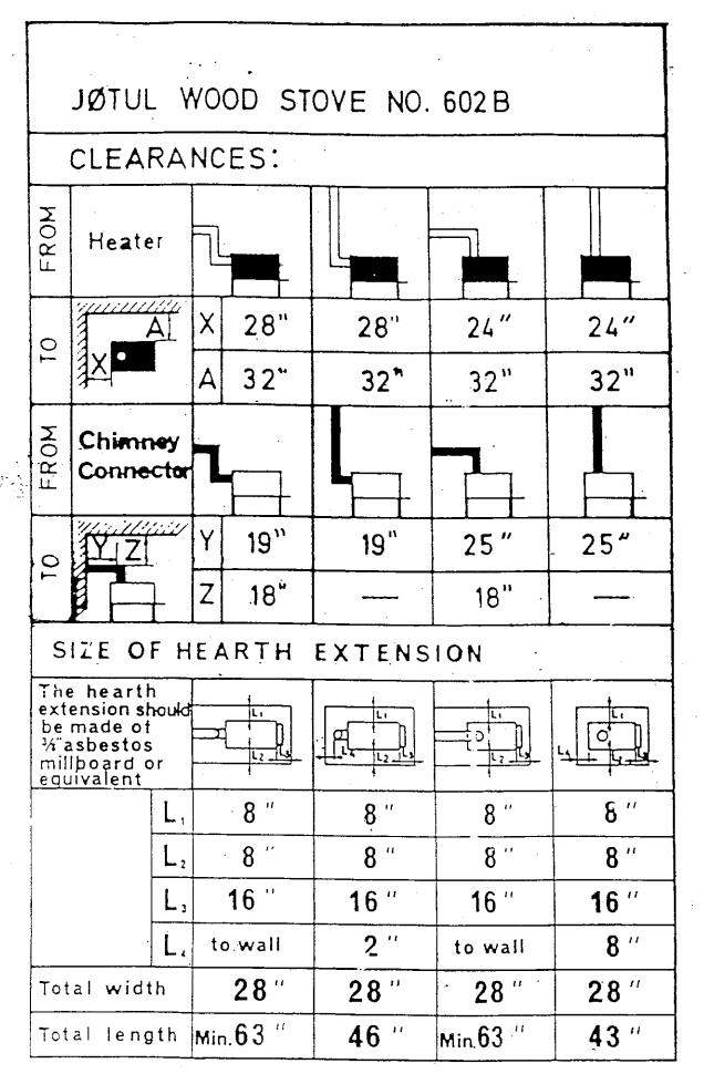
Fig.1 Clearances and Hearth Extension Size
