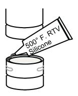
Seal each vent section by applying a liberal amount of 500°F RTV silicone around the gap between sections.
