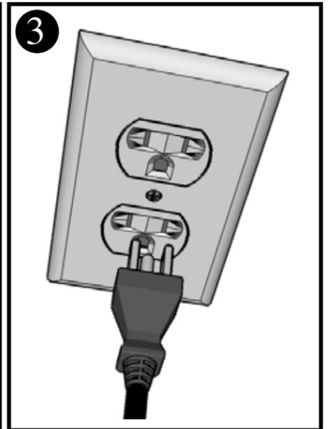
Plug into a grounded three-pronged outlet. The DRAW COLLAR runs at 120V, 500 Watts.
