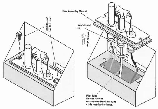
Remove the pilot orifice. It may be resting on the pilot tube or lodged inside the pilot assembly (tap the asembly from above until it falls out). Place the propane pilot orifice onto the pilot tube (the LP orifice is .016" diameter - it has "16" stamped on it). Insert the pilot tube (with orifice) into the pilot tube port and tighten the compression nut until tight. NOTE: Leak test this connection after the heater is installed and gas is connected.
