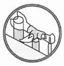
The pilot flame must contact the thermopile and thermocouple (see the illustration to the left). If it does not, turn the gas control valve to "OFF" and call your dealer.
