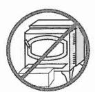
• It is imperative that control compartments, screens, or circulating air passageways of the heater be kept clean and free of obstructions. These areas provide the air necessary for safe operation.
