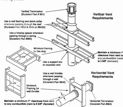
• Use Model GS Direct Vent manufactured by Simpson Dura-Vent only (or the Chimney Conversion Kit - see Addendum #2). Follow the installation instructions included with the vent. For the nearest Simpson Dura-Vent supplier, call (800) 835-4429. Part numbers and descriptions are listed below.
