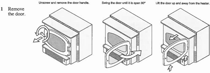
NOTE: When re-installing, make sure the handle points away from the glass when finished.
