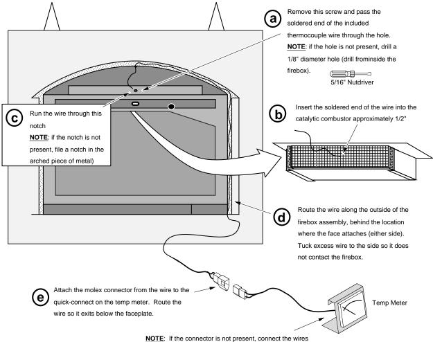
**NOTE:** If the connector is not present, connect the wire to the two posts on the back of the temp meter. The yellow inner wire goes to the positive (+) pole.
