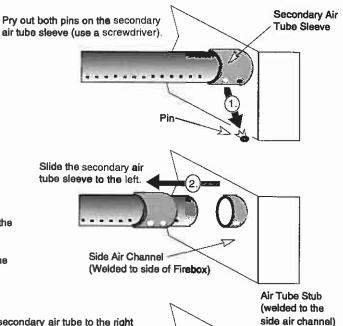
NOTE: When replacing, make sure the two holes on the secondary air tube sleeve line up with the hole on the secondary air tube and the hole on the air tube stub welded to the side air channel.
