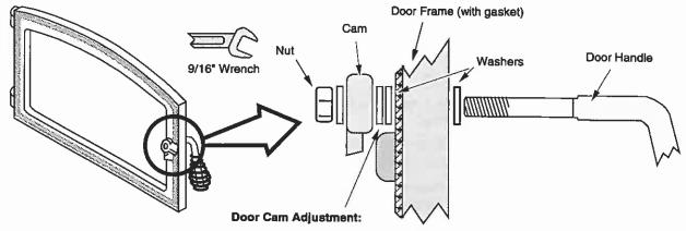
To tighten the door cam, remove the door handle and discard one of the washers between the door frame and cam. To loosen the door cam, add a washer between the door frame and cam.
