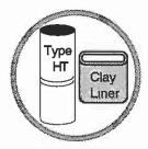
This appliance must be connected to a listed high temperature (HT) residential type chimney or an approved masonry chimney with a standard clay tile, or stainless steel liner.
