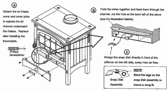
3 Install the wire clip following the directions below.
