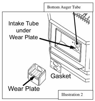
obstructions in the tube under the wear plate. Check for any build-up in the front of the burn area. Clean out all air holes (if necessary a 1/8" drill bit can be used) --these air holes should be kept clean, as they supply combustion air under and around the pellet fuel. The burn pot assembly should also be thoroughly cleaned, including the burn box. When replacing the wear plate, ensure that it lies flat in the firebox and no gaps (from ash residue) are under it.
